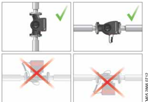
Fig. 10 Installation positions
