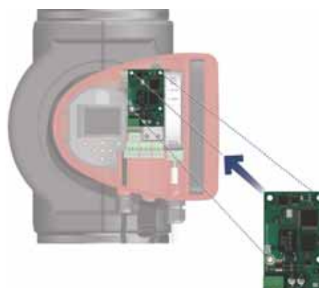
Fig. 58 Location of CIM module
