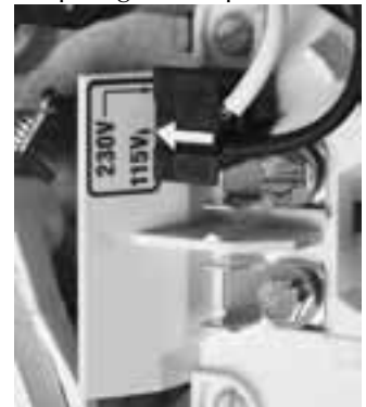
Figure 4B - Voltage Change Plug Set for 115 Volts
