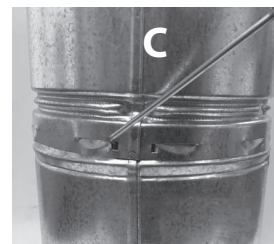
To disengage the DuraLock, pull out all lances (teeth). Rotate joint slightly while gently pulling apart.
