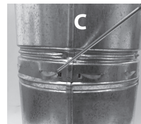
To disengage the DuraLock, pull out all lances (teeth). Rotate joint slightly while gently pulling apart.
