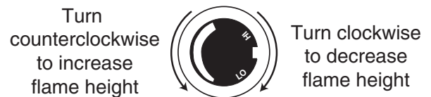
Fig. 30 Flame adjustment knob for SIT valve.
