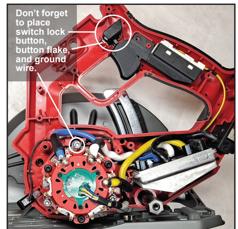
Follow directions in reverse order to put assembly/tool back together. Be sure there are no interferences and wires are properly placed within traps/channels.
