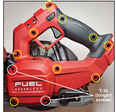
Remove from left housing/handle nine T-15 screws (fig.63) circled in yellow, two T-10 screws (fig.67) circled in white and one T-8 screw (fig.78) circled in green.
