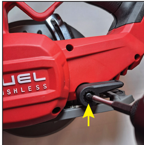
Remove T-25 screw (fig.69) from inside plunge lever.
