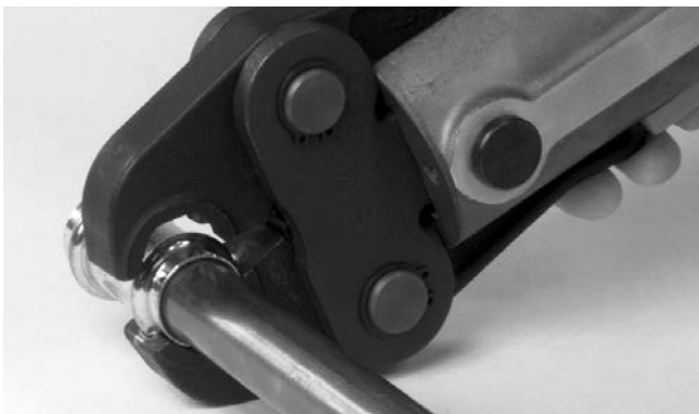
Figure 10 – Opening the Jaw set and Placing Around Fitting
