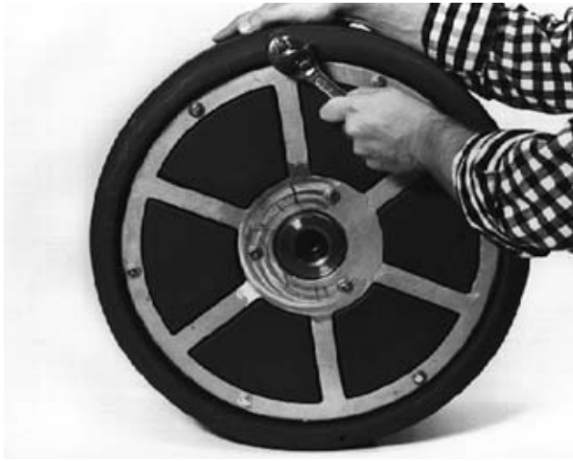
Figure 23 – Removing Pigtail Anchoring Bolt
